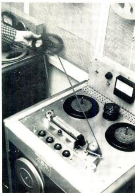
Figure 3. Extending the loop length and placing it through an empty 7-inch plastic reel.
